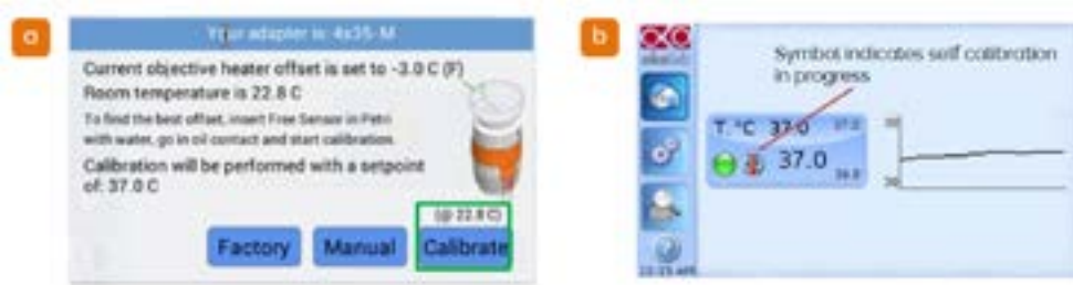
Figure 76: a) Tap on Setting > Temperature > Objective Heater and Calibrate. Then Start. b) The calibration procedure typically takes more than one hour. When the calibration is in process, a reminder icon will appear on the Temperature tab. Once completed, the icon will disappear.
