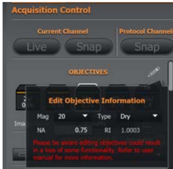
Figure 97: Enter the objective lens magnification (Mag), numerical aperture (NA), and type (Dry or Oil) of the new objective lens. An objective lens' magnification and numerical aperture can always be checked and verified in the engravings on the side of the objective lens barrel that is being installed.
