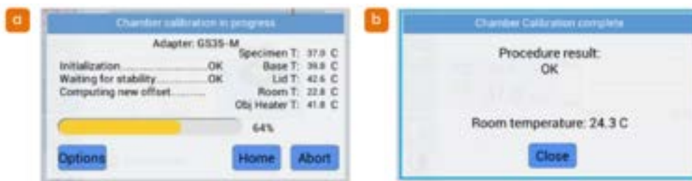
Figure 74: a) The system will automatically start the calibration procedure and show a progress bar, calibration may take 1-2 hours to complete. b) Once the self-calibration procedure is complete, the window shown will be displayed.
