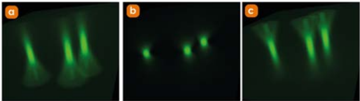
Figure 106: When the correction collar is correctly set to a value that matches the thickness of the sample's coverslip spherical aberrations are reduced and a symmetrical response is observed above and below the sample volume. In the above example a sample containing 1 \mu\text{m} beads mounted on a standard 170 \mu\text{m} coverslip is imaged at 40x to obtain a z-stack with the correction collar set at a) 110 \mu\text{m} b) 170 \mu\text{m} and c) 230 \mu\text{m} . When the correction collar value is set too low (a) or too large (c) the asymmetric nature of the 3D image is clearly visible; when set at the correct value for the sample (b) the best quality image is produced.
