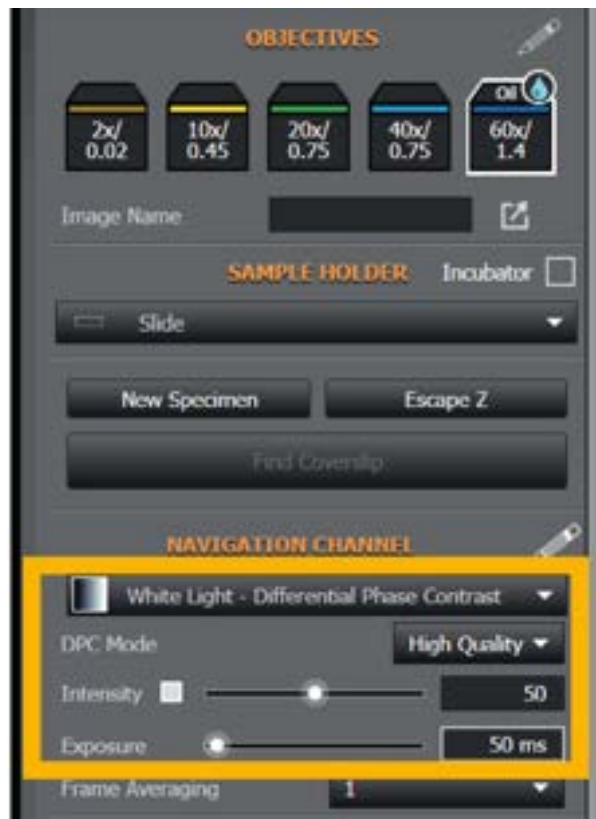
Figure 161: Change the Navigation Channel to the Differential Phase Contrast channel. Set the Exposure time to 50 ms and choose the High Quality Mode.
