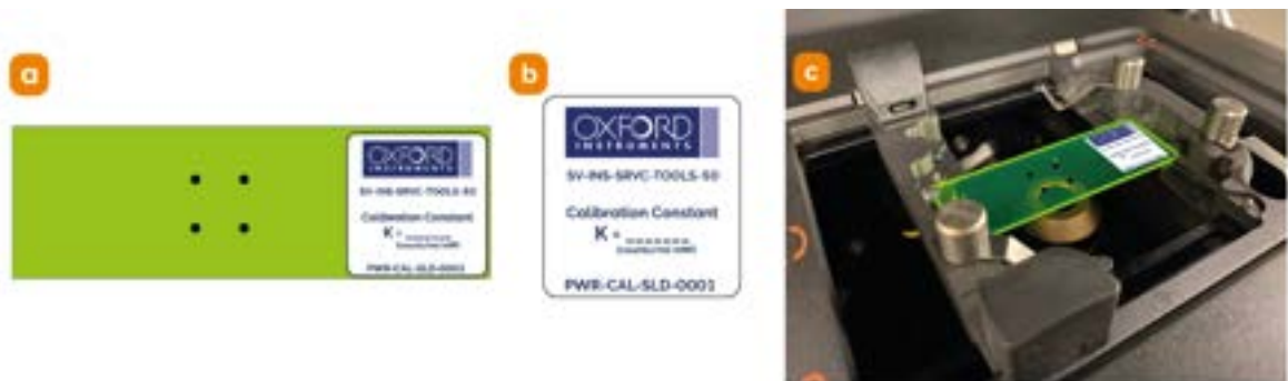
Figure 169: a) Obtain the calibrated green fluorescent plastic slide. b) Note the full serial number code associated with this slide of the format PWR-CAL-SLD-####, where #### is a 4-digit number. Also note the calibration constant, K, written on the slide label. c) Lift open the top cover lid of microscope, load the green plastic slide into the sample holder as shown, and then close the top cover lid.
