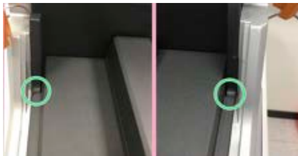
Figure 130: Ensure the XY stage is centred by looking at the rear corners where the XY stage meets the rear chassis. Both sides should be flush.
