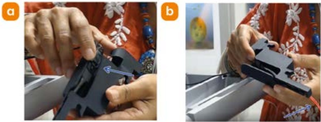
Figure 60: a) Fit the terminal end of the objective heater cable connector into the objective heater cable holster. b) The orange cable leading to the wrap-around heater should hang out of the shaft end of the holster. Now reinsert the holster back into the front chassis of the BC43.
