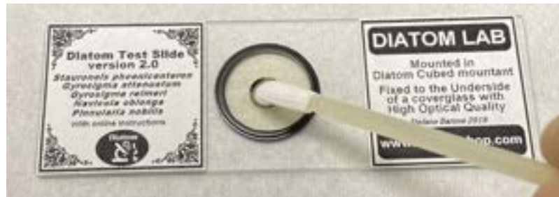
Figure 152: Apply a few drops of optical grade lens cleaning solvent to tip of a cleaning swab. Thoroughly clean the coverslip surface and the backside of the slide within the black encircled area of the sample using an outwardly spiralling motion of the swab in contact with the glass surfaces.
