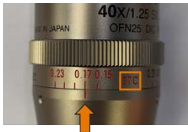
Figure 105: If you are imaging your specimen in a 37 degree heated environment such as the Okolabs stage-top incubator (H301-K-FRAME-AD), check if your objective lens has a correction collar scale for this temperature and use this scale instead of the room temperature scale.
