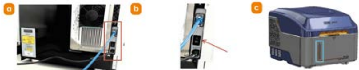
Figure 77: a) and b) Turn the power switch located on the lower-right corner of the back panel to the ON position. BC43 will undergo its start-up sequence. c) The LED on the front panel will flash a blue light. Once the blue LED light is stable BC43 is ready to be connected to the Fusion control software.
