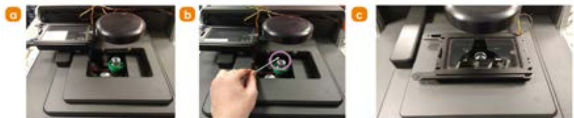
Figure 68: a) Carefully set the imaging chamber aside. b) Use a solvent-soaked cleaning swab or lens tissue to wipe the oil from the oil immersion objective lens. c) Carefully re-insert the stage-top live-cell imaging chamber into the XY stage.
