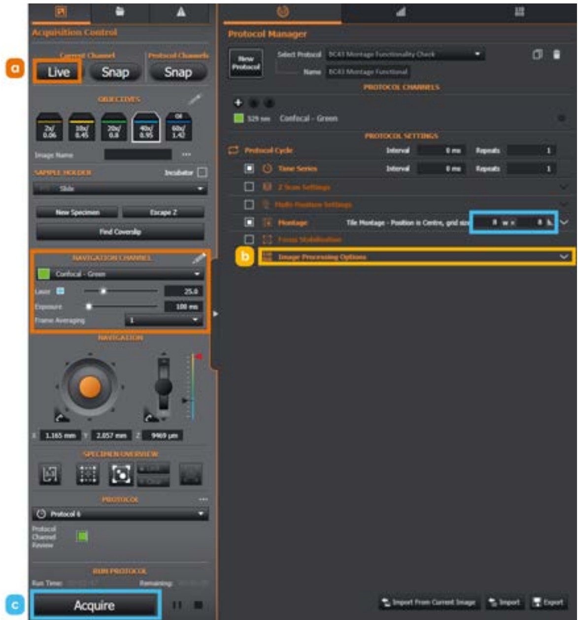
Figure 163: a) Click Live and finely adjust the focus to midplane of the cellular specimen using the Confocal - Green channel. b) Once the protocol is imported navigate to the Image Processing Option area and ensure Stitching is set to ON. c) Click "Acquire" in the Protocol Manager to capture a 8x8 stitched montage of the specimen.
