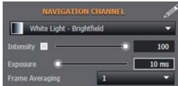
Figure 146: In the Fusion remote panel, under the Navigation Channel heading, activate the Brightfield channel. Set the transmitted LED turret Intensity to 100%. Set the Exposure time to 10 ms.
