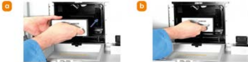
Figure 120: With one hand holding the Focus Seek and Lock module front handle and the other hand holding the front frame of the module, carefully guide the device back into the front chassis. When the replacement module is almost fully inserted, apply slight pressure, and the module pins and magnets should click into place.
