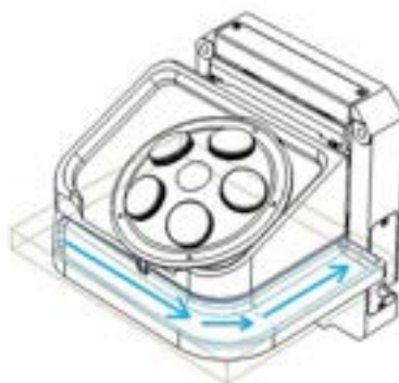
Figure 107: The image shows the motorised objective turret and Z-stage installed in the unit. The drip tray is highlighted in blue.
