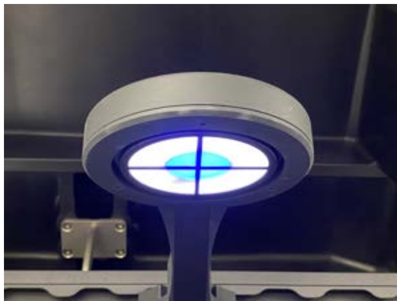
Figure 147: With the top cover lid open, squat down and observe the underside of the transmitted light turret from a distance at an oblique angle. Verify that outer annulus of the LED turret is constantly ON and has a white colour as shown. Also verify that the central section of the LED turret is constantly ON and exhibits a blue colour as shown.
