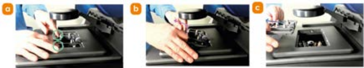
Figure 35: a) Grab hold of the front edge of the sample holder with two hands. b) Pull up and away to release the sample holder from the sample stage. c) Fully remove and set aside the sample holder.
