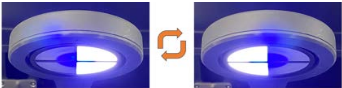
Figure 149: With the top cover lid open, squat down and observe the underside of the transmitted light turret from a distance at an oblique angle again. Verify that LED turret rapidly alternates turning ON/OFF the left/right halves of the turret.
