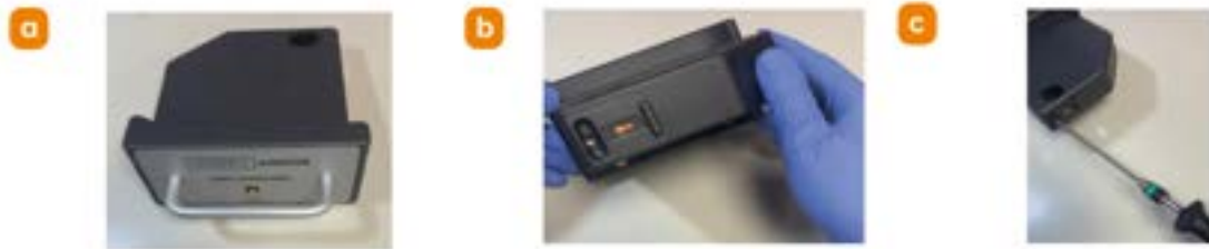
Figure 110: a) Turn the removed Focus Seek and Lock module around to its backside and locate the dichroic mirror mount locking setscrew. b) The orange arrow on the back of the module points to this setscrew. c) Unscrew the mirror mount from the module using the T20 Torx bit loaded into the 1.2-3 Nm Torque Gun.
