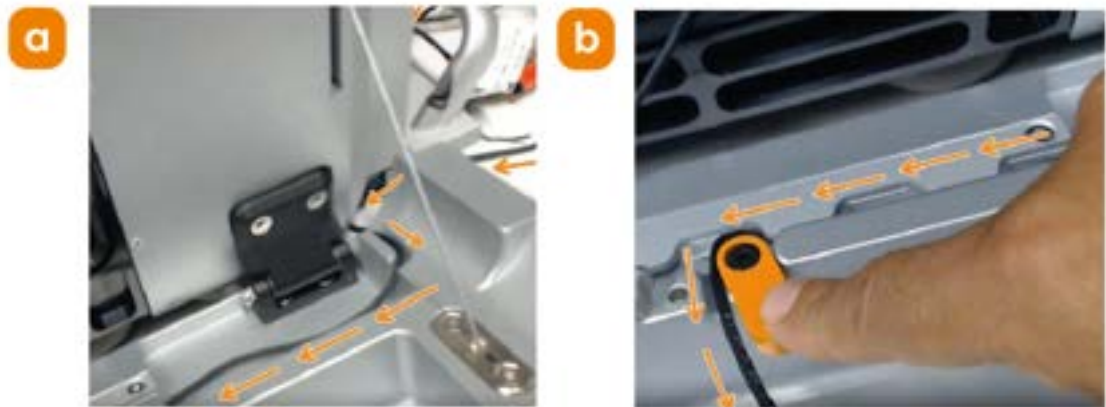
Figure 59: a) Route the objective heater cable through the lower-left corner of the BC43 unit and feed the cable through the grooves in the backside of the front panel access door. b) Bring the cable to the middle of the backside of the door and pass it under the orange swing-out latch. Close the latch once the cable is through.
