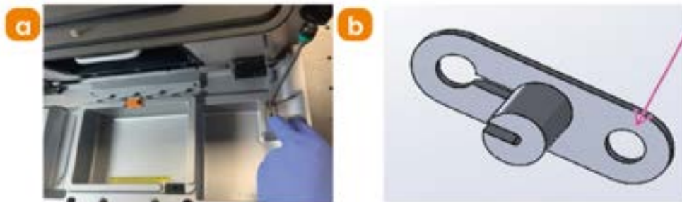
Figure 138: Attach the drawbridge mechanism facet to the backside of the replacement door with two screws using the T20 T-Shape Key. Ensure the circular through-hole of the facet is positioned with the screw hole as shown.
