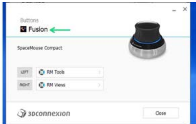
Figure 23: Check the Fusion logo appears as shown in image. If it does not, check that Fusion is running and relaunch the 3Dconnexion app.
