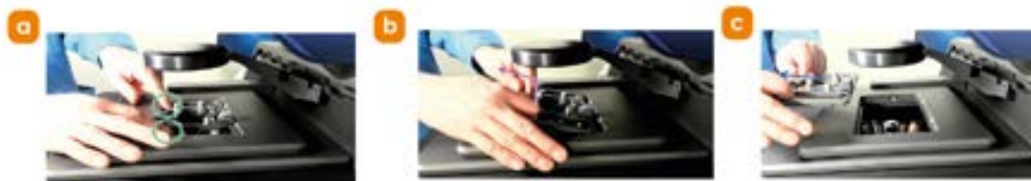
Figure 78: a) Grab hold of the front edge of the sample holder with two hands. b) Pull up and away to release the sample holder from the stage. c) Fully remove and set aside the sample holder.
