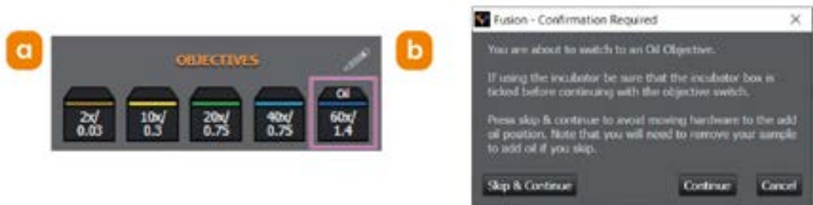
Figure 63: a) Click on the oil objective lens icon. b) A message prompt will appear confirming the selection to switch to an oil immersion objective. Click 'Yes' to continue.
