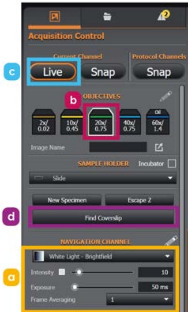
Figure 154: a) In the Fusion remote panel, under the Navigation Channel heading, select the Brightfield channel and set the Intensity to 10% and the Exposure time to 50 ms. b) Activate a low magnification objective lens compatible with the Find Coverslip software feature such as a 20x air objective. c) Click the Live button to activate the live preview. d) Click the Find Coverslip button to automatically find focus on the test slide coverslip.
