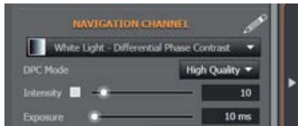
Figure 150: In the Fusion remote panel, under the Navigation Channel heading, activate the Differential Phase Contrast channel. Choose the High Quality mode. Set the transmitted LED turret Intensity to 10%. Set the Exposure time to 10 ms.
