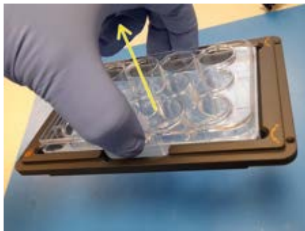
Figure 94: With the wellplate located in the multiwell frame gently grab the wellplate and lift up. If this action also lifts the multiwell frame the assembly is complete.
