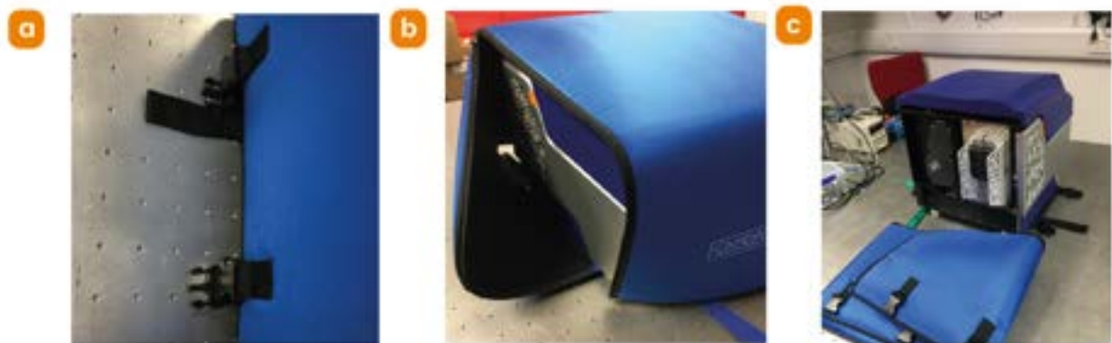
Figure 17: Removing the dust jacket on BC43. a) Unclip the side straps. b) Unzip the side panel. c) Remove the dust jacket.
