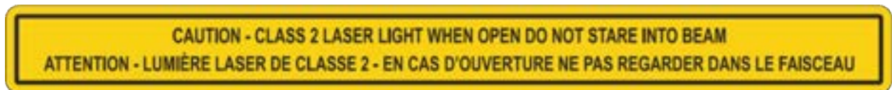
Figure 4: Label located adjacent to the top lid on the front door panel.
