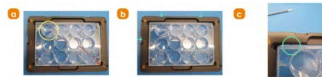
Figure 93: a) Multiwell plate inserted in multiwell plate holder with A1 well in top-left position. b) and c) While still pushing against the sides of the multiwell plate, turn in the three adjustable setscrews with the 1.5 mm hex driver until the ball end of each setscrew is in light contact with the side wall of the inserted multiwell plate.
