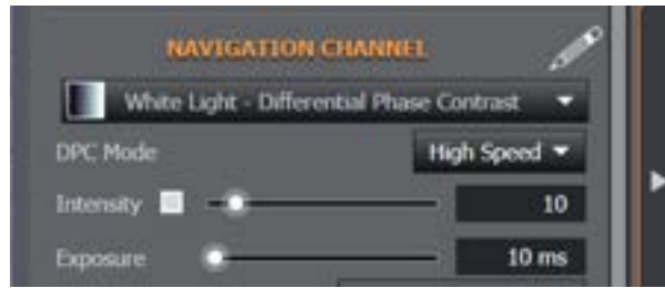
Figure 148: In the Fusion remote panel, under the Navigation Channel heading, activate the Differential Phase Contrast channel. Choose the High Speed mode. Set the transmitted LED turret Intensity to 10%. Set the Exposure time to 10 ms.
