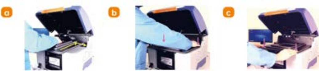
Figure 129: a) Grab hold of the new stage to be inserted and guide it under the transmitted light turret and then tilt the back edge downwards into the recess adjacent to the left and right-side cosmetic panels. b) and c) Apply downward pressure onto the back and front corners of the stage, while checking from the side to see if the stage fits into its space and that the stage pins located on the underside of the lower-left corner have made good contact with the blind mate connectors.
