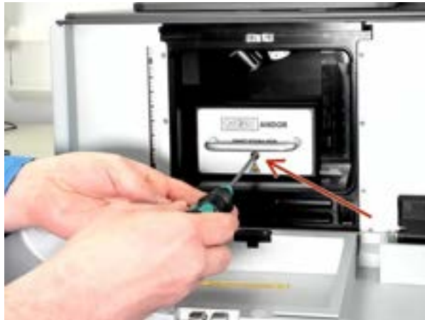
Figure 117: Using the T20 Torx bit loaded into the Adjustable Torque Screwdriver 1.2 - 3 Nm, loosen the front captive screw to unlock the Focus Seek and Lock Module.
