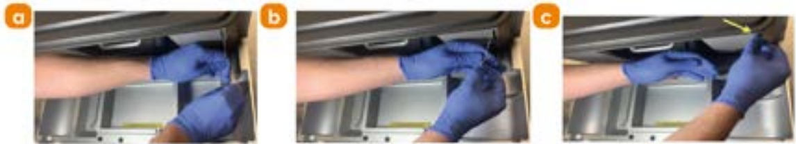
Figure 133: With both screws now removed, grab hold of the drawbridge mechanism facet and let the cord recoil (while still attached to the facet), and rest it against the front panel.
