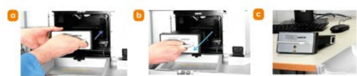
Figure 118: a) Grab hold of the Focus Seek and Lock module handle. b) Ensure to use two hands, one at the front and one to support the module as you slowly pull the Focus Seek and Lock Module straight back and outwards until it is completely free of the front chassis.
