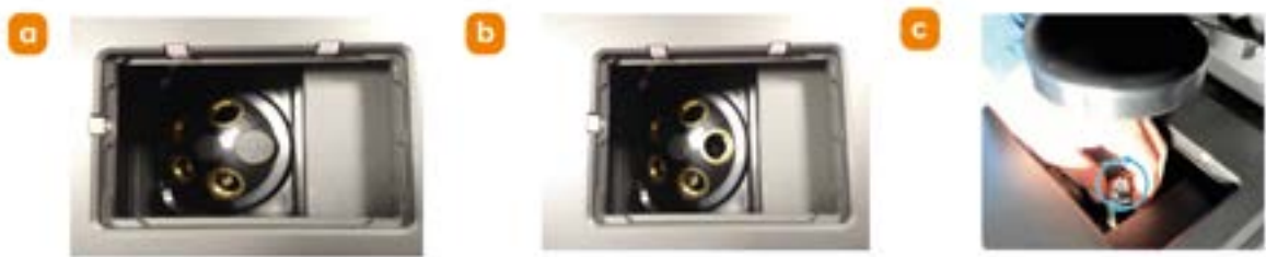
Figure 37: a) Empty objective turret with nosepiece cap. b) Empty objective turret with nosepiece caps removed. c) Turn the objective clockwise to install.
