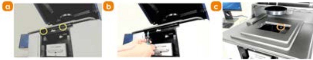
Figure 131: a) and b) loosely screw in the front XY stage hex screws (do not tighten at this stage) and c) the rear captive screw using the 1.2-3 Nm torque gun. Now tighten the rear captive screw, torque set to 3.0 Nm. Now go back and tighten the loose front screws to 3.0 Nm.
