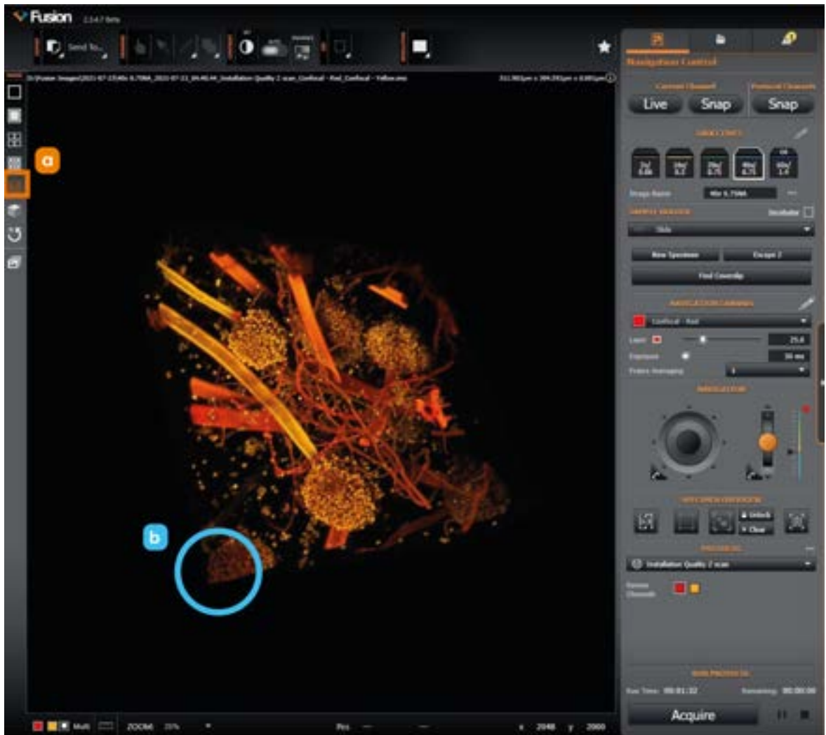
Figure 168: a) Click on the 3D Maximum Intensity Volume view. b) With the mouse, left-click and grab hold of the 3D rendered image of the fungus and rotate it around in 3D space. Closely examine the result of 3D reconstruction move around to see if there are any obvious regions where the rendering has failed to display properly.
