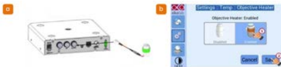
Figure 75: a) Keep the petri dish with the green sample probe in the chamber. Check that the objective heater has been correctly connected to the temperature control unit and secured to the objective of choice. b) Check that the objective heater is enabled by
