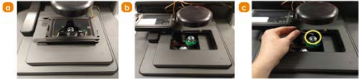
Figure 65: a) and b) remove Okolab incubator. c) Apply a small drop of immersion oil onto the top lens of the oil immersion objective lens.
