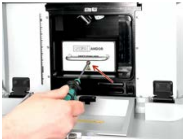
Figure 121: Using the T20 Torx driver, tighten the front captive screw to lock the Focus Seek and Lock module into the front chassis. Torque to 2.2 Nm.
