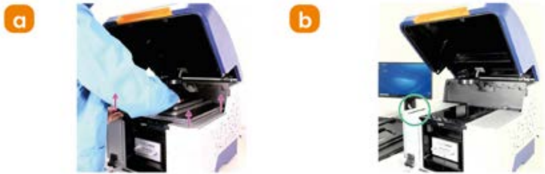
Figure 127: a) With the front screws and rear captive screw backed off, grab hold of the stage with one hand through the sample holder and nudge up the lower left corner to release the stage from the blind mate connectors. When the stage is free of the chassis, carefully pull it away from the unit, being careful not to crash or knock the transmitted light illuminator. b) Note the exposed stage bind mate connectors.
