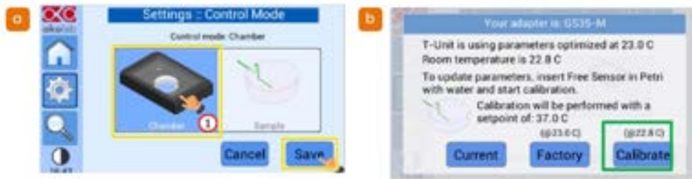
Figure 73: a) Tap Settings > Control Mode > Chamber > Save. b) When the calibration dialog appears, tap on Calibrate.
