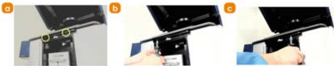
Figure 125: a) Location of chassis screws. b) Unscrew first and c) second screws.
