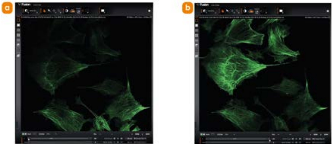
Figure 81: Poor sample tilt. a) Z plane: 20. b) Z plane: 25. Different areas of the monolayer sample come into focus at different positions in the Z plane.
