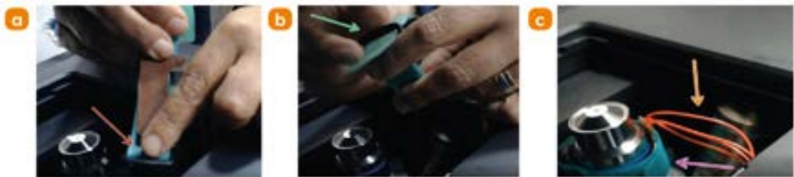
Figure 61: Secure objective heater band to immersion objective lens. a) Position the brown heater band within the blue velcro strap such that there remains about one fingernail size of space between the ends of the two straps. b) Feed one of the velcro strap into the black buckle on the other end to make a loop. Loosely pull the band loop over the immersion objective lens to its mid-section, then pull on the green velcro strap to tighten around the objective and press down the free end of the tightened strap. c) The orange cables of the objective heater should comfortably be slacked and feeding to the shaft of the objective heater cable holster.
