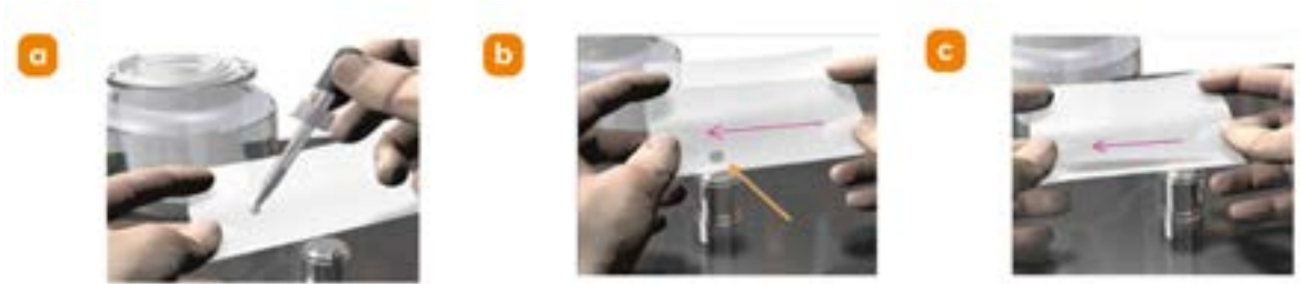
Figure 108: a) Place a drop of Sparkle Lens Cleaner or equivalent lens cleaning solvent on a single piece of lens tissue. b) and c) Lay the wet portion of the lens tissue on the top lens of the objective, then slowly pull the tissue to the left until the drop streak completely dries.
