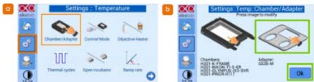
Figure 71: a) From the controller touch screen, tap Settings > Chamber/Adapter. b) Select the correct insert by tapping the screen until the correct insert appears. Tap OK.
