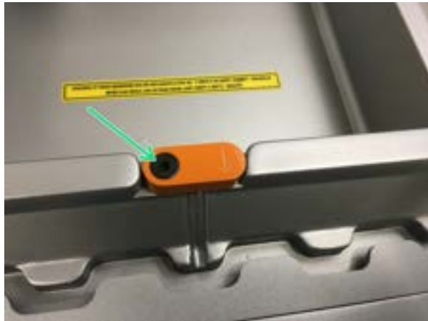
Figure 140: Unscrew the touch latch using 2.5mm Hex bit loaded into the AdjTorqGun 0.3 - 1.2 Nm.
