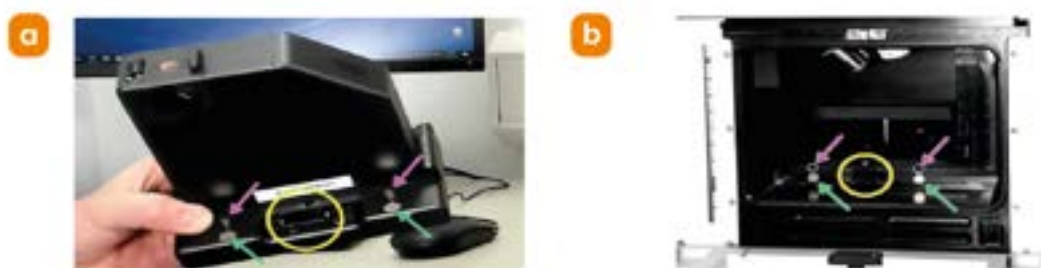
Figure 119: Note the following features on the underside of the Focus Seek and Lock module: (quantity 2) magnets (quantity 2) guide pins, the module's blind-mate electrical
