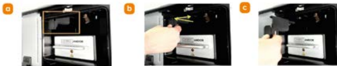
Figure 122: a) The objective heater cable holster is located on the upper-left corner of the front chassis left wall which is now accessible through the front access panel door opening. b) Grab hold of the lower end of the holster with one hand and pull back towards the front of the instrument to release the holster from its locator pins. c) Then pull the holster to the right to remove from the front access door panel opening.
