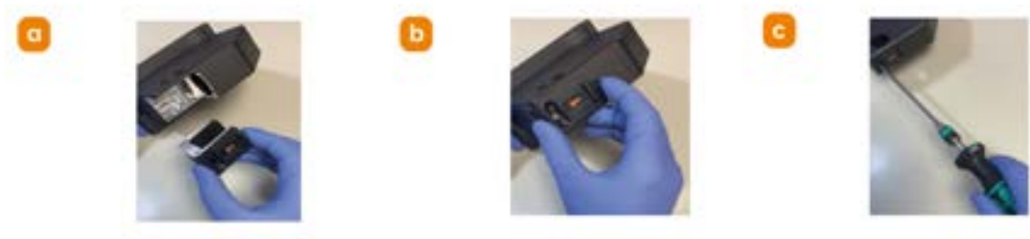
Figure 114: Fit the dichroic mirror mount back onto the Focus Seek and Lock module and lock in by tightening the setscrew with the T20 Torx bit loaded into the 1.2-3 Nm Torque Gun.
