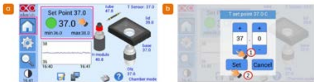
Figure 72: a) Go back to the home-page, and b) set the temperature to 37.0°C
