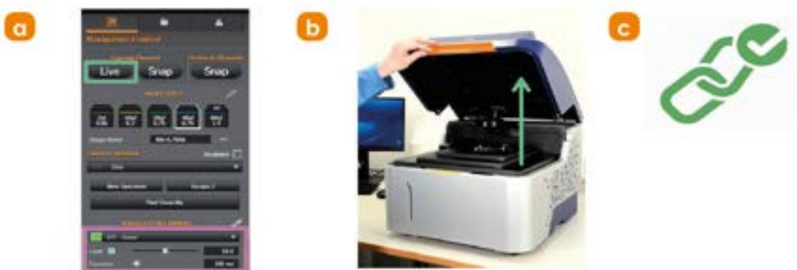
Figure 139: a) In Fusion, activate the EPI - Green channel. Set the laser power to 50%. Set the exposure time to 100 ms. Click "Live", and then fully open the top cover lid. b) After 5 minutes of being open, the laser will stop emitting and will not resume until the lid is closed and opened again. c) Observe the blue laser light emitting from the objective lens, and verify that the interlock activates after 5 minutes, is shutting off the laser light completely.
